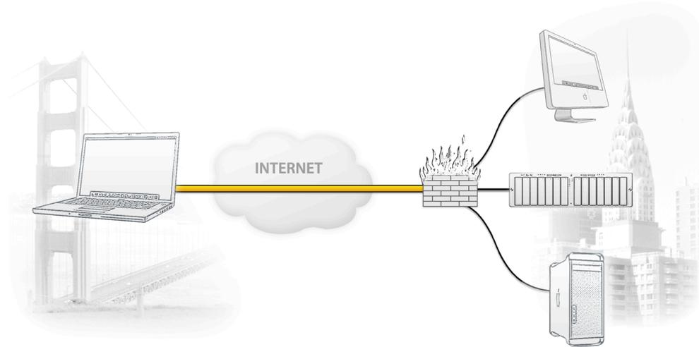
The MacBook is directly connected to the Internet and has a public IP address, assigned by an ISP.
